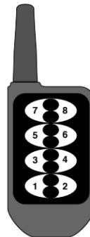
**Button 1** Spray on demand. A spray cycle activates for the length of the programmed spray duration (**pressing button 1 again during the spray cycle will end the current spray cycle immediately**). The system reverts back to pre-programmed settings after each spray.
